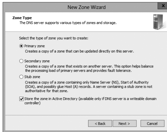
FIGURE 3.6 Setting up an Active Directory Integrated zone
