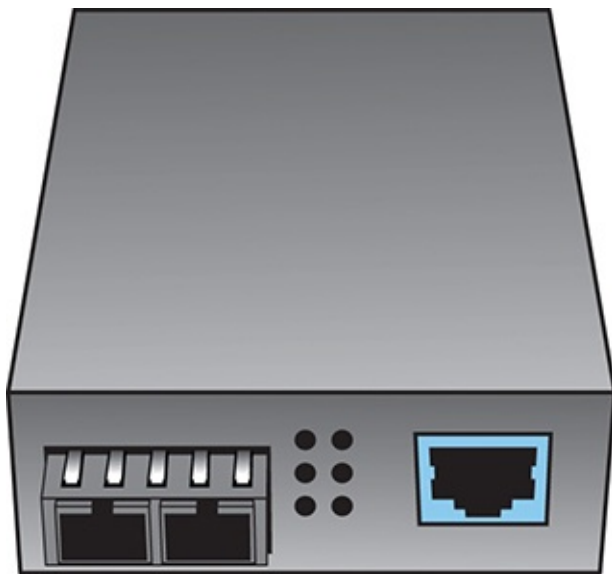
FIGURE 4.3 A common media converter
