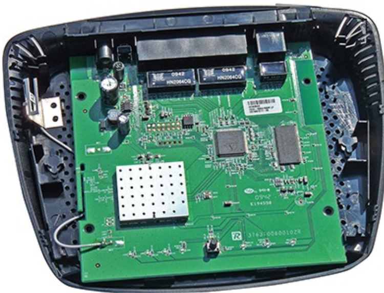
FIGURE 7.2 The antenna is the wire and metal component on the left
