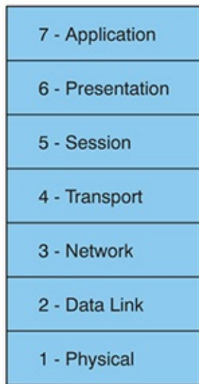
FIGURE 2.1 The OSI seven-layer model
