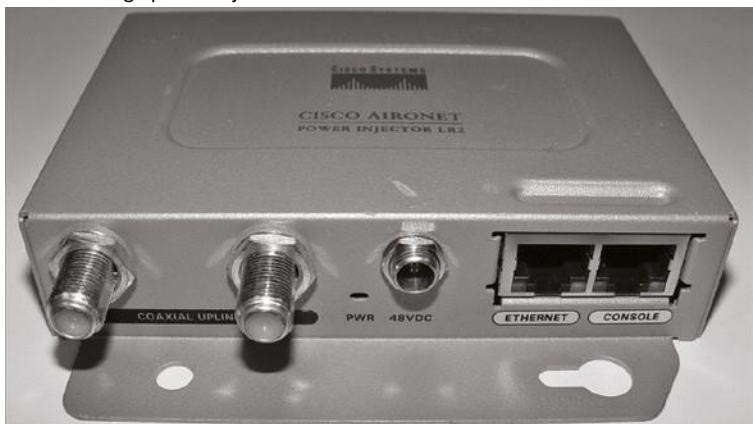
FIGURE 11.25 Wireless bridge power injector
