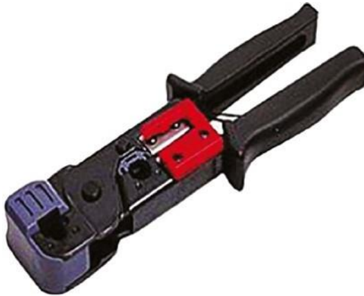
FIGURE 23.11 A combination cable stripper, crimper, and snippers
