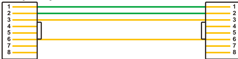
FIGURE 3.21 Straight- through Ethernet cable
