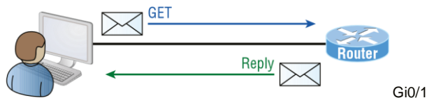
FIGURE 22.1 SNMP GET and TRAP messages
