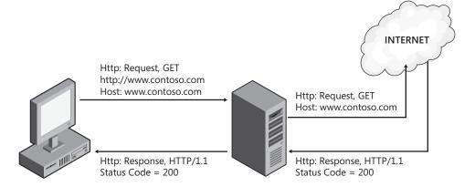
FIGURE A-4 The proxy sends the request to the Internet server on behalf of the client.
