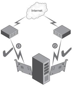
FIGURE 5-9 ISP load-balancing
