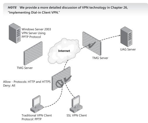
FIGURE 2-1 Comparing SSL VPN with the traditional VPN
