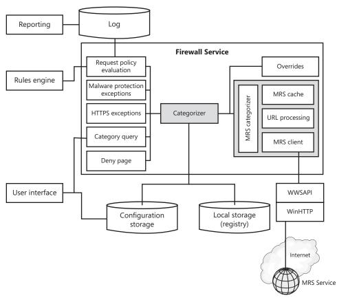
FIGURE 18-3 Components that are affected by URL Filtering process
