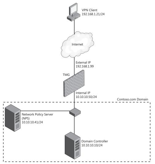
FIGURE 26-18 Topology used in this scenario to configure Forefront TMG with NAP Integration
