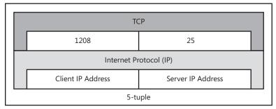
FIGURE 21-5 Packet destined to a route-based Server Publishing rule
