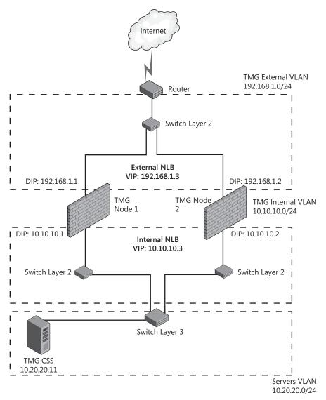
FIGURE 13-44 TMG CSS located in a non-array member
