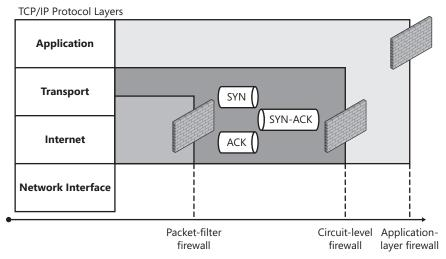
FIGURE 1-4 The three main firewall generations
