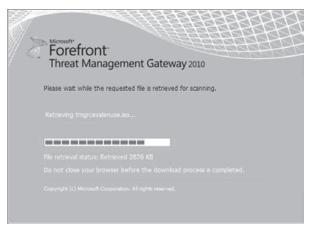
FIGURE 1-6 An HTML page displayed to the client while inspection takes place
