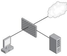
FIGURE 2-5 TMG as 3-leg perimeter firewall
