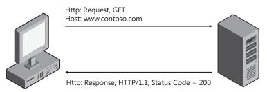
FIGURE A-2 Basic communication between client and server using HTTP Protocol
