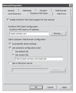
FIGURE 6-4 Internal network configuration
