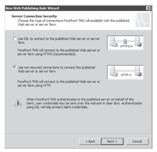
FIGURE 22-13 Selecting the protocol that the internal Web server will use
