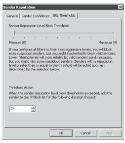
FIGURE 19-45 Configuring the sender repudiation threshold
