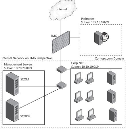
FIGURE 17-5 Reference topology diagram
