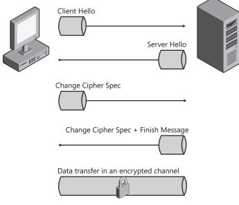
FIGURE 32-2 SSL handshake phases
