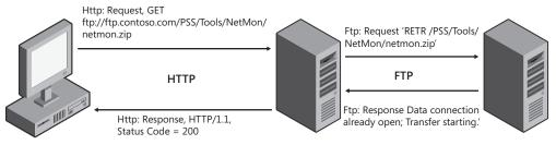
FIGURE A-5 How CERN proxy handles a FTP request
