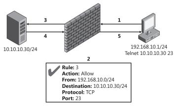
FIGURE 1-3 A packet-filtering firewall using basic access control lists
