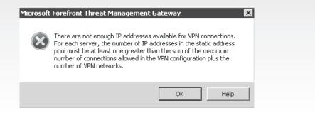
FIGURE 27-17 Insufficient address range warning
