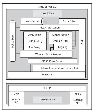
FIGURE A-7 Proxy 2.0 functional architecture
