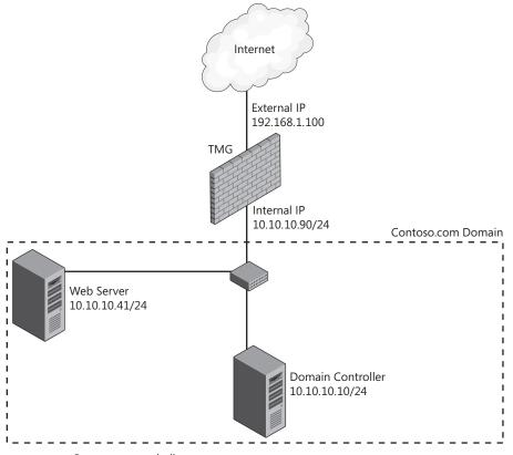
FIGURE 22-1 Contoso network diagram
