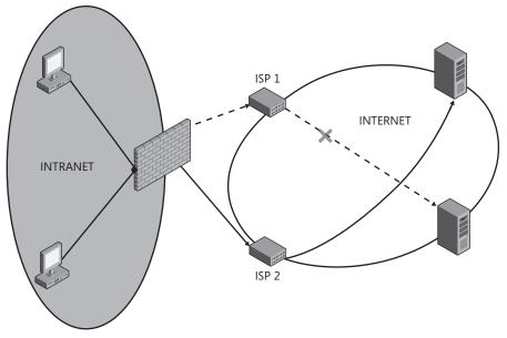
FIGURE 13-1 The ISP Redundancy feature in TMG
