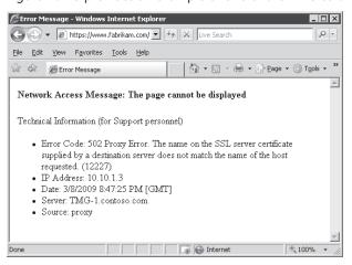
FIGURE 20-25 TMG Certificate Validation Failure
